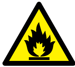
Flammable material or high temperature*
