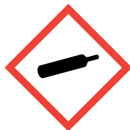
Gas under pressure
