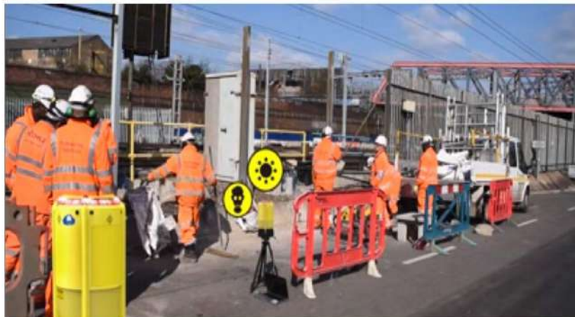
It monitors environmental factors - like dust, UV, noise, and radiation, and location
